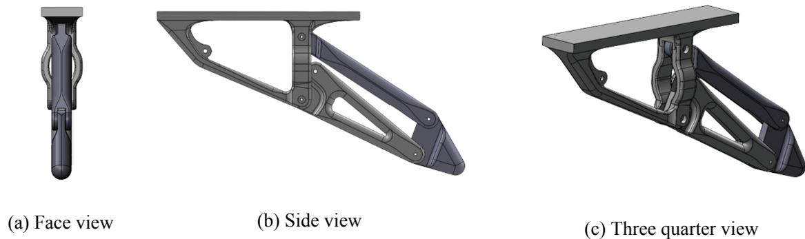
Fig. 5-10 General assembly views of the mechanical landing gear
